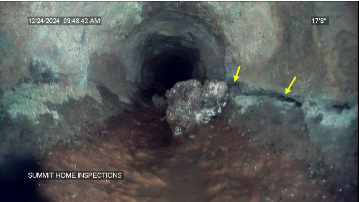
cracked cast iron under house
